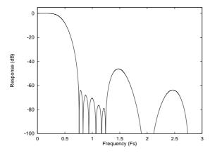
Figure 25 ADC Digital Filter Frequency Response – Type 2
