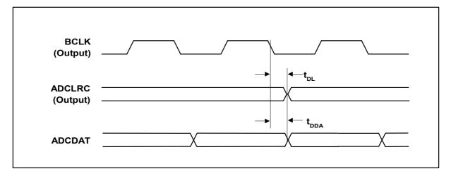
Figure 3 Digital Audio Data Timing – Master Mode
