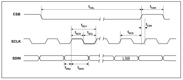
Figure 6 Program Register Input Timing – 3-Wire MPU Serial Control Mode
