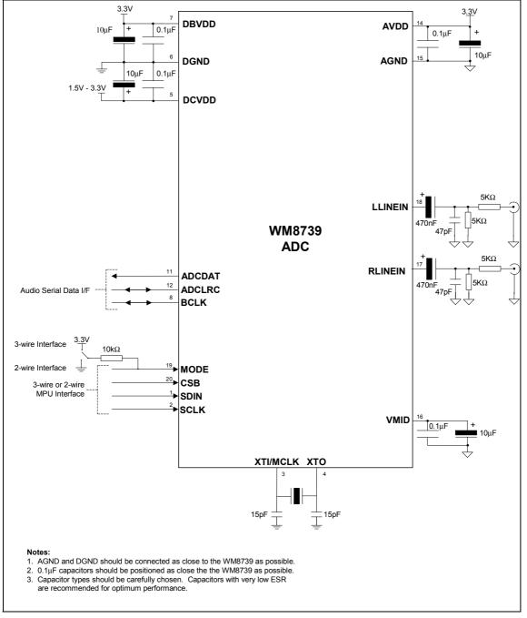
Figure 29 External Components Diagram
