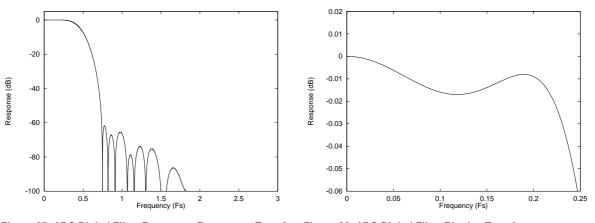
Figure 27 ADC Digital Filter Frequency Response – Type 3
