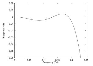
Figure 26 ADC Digital Filter Ripple – Type 2
