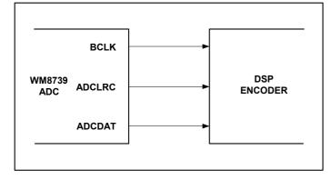
Figure 2 Master Mode Connection
