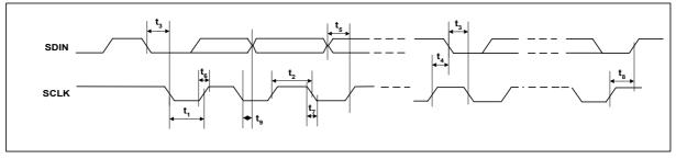
Figure 7 Program Register Input Timing – 2-Wire MPU Serial Control Mode
