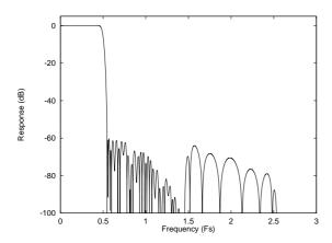
Figure 23 ADC Digital Filter Frequency Response – Type 1
