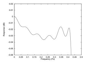
Figure 22 ADC Digital Filter Ripple – Type 0
