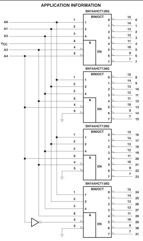
Figure 3. 32-Bit Decoding Scheme
