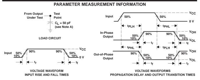
NOTES: A. CL includes probe and test-fixture capacitance.
