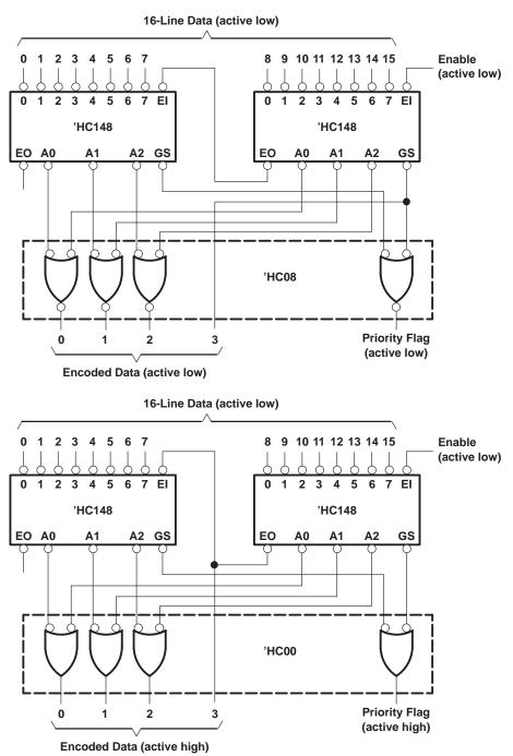
Figure 2. Priority Encoder for 16 Bits
